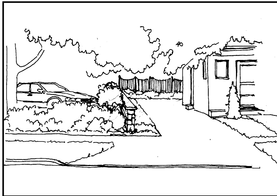
Sketch 2: A continuous evergreen landscape buffer and a masonry wall at the property line.
